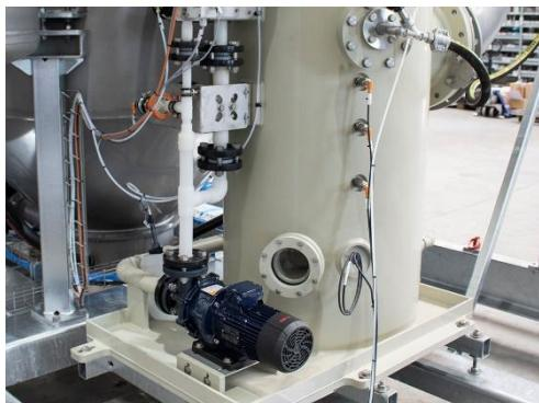
Components for sulphuric acid and vapour scrubbers made of **stainless steel** as well, thus durable and no corrosion.
