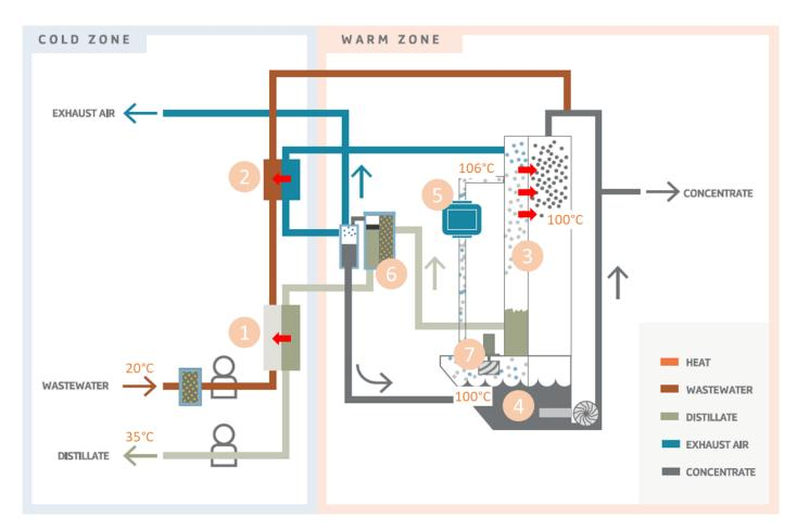
The slurry goes through three heat exchanger (1,2 & 3) to the process tank (4). Here it is circulated and heated by the main heat exchanger (3).
