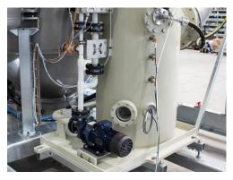
Components for sulphuric acid and vapour scrubbers made of **stainless steel** as well, thus durable and no corrosion.
